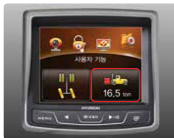
Load Indicator A load can be placed on the fork and can be accurately weighed by measuring the hydraulic pressure.
